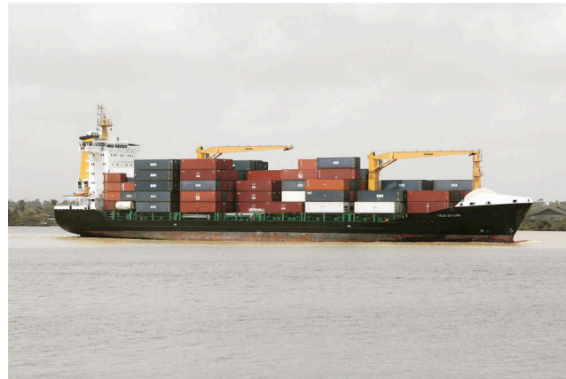
3.56 This container ship, which is navigating the Suriname River on its way to the port of Paramaribo, Suriname, is an example of the type of highly mechanised vessel that can operate with a minimal crew to maximise profitability. The large cranes visible on the ship can be operated by a few individuals, thus keeping costs to a minimum while maximising the rate at which large quantities of freight can be loaded and unloaded.
