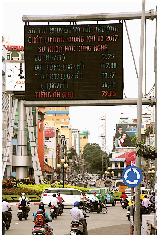
8.19 Measuring roadside air pollution and noise levels in Ho Chi Minh City, Vietnam. Continual monitoring of air pollution is conducted along roads by automated sensors that send data to a central processing monitoring centre. This display rotates through different measures, including carbon monoxide, dust, nitrous oxides and acidity.
