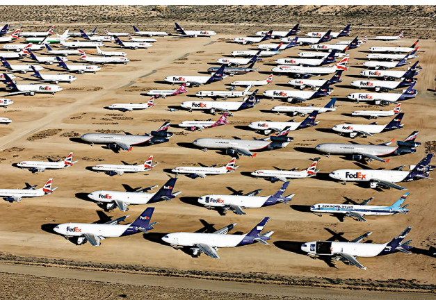
2.57 When airliners reach the end of their service lives, they are often stored in desert environments such as this aircraft graveyard in Victorville, California, USA, where the dry climate is less corrosive on metal components than more humid areas. The three aircraft nearest the camera in this view are Airbus A310 freighters, with various parts already cannibalised for use on aircraft that are still flying.
