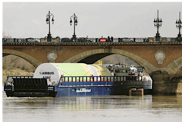
2.56 Parts of the first production A380 on a river barge passing under the oldest bridge in Bordeaux. This hazardous operation can only be performed at low tide because of the low clearance of the bridge. Tracks around the bridge pillars have been set in place to protect them from damage by the barge.
