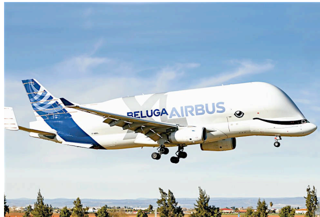
2.54 A Beluga XL freighter, specially built to carry large components between suppliers and Airbus assembly plants, seen here flying from Spain to the large Airbus factory in Toulouse, France.
